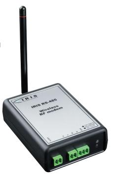
The unit can create and send both fixed text string and strings with parameters. The parameters can for example contain the unit's id or alias, the received text, status of logical flags, RSSI and values of timers and counters. The created text messages can be sent as commands to other units or as information to the user. There is a special command that changes the value of the logical flags and outputs on other units.
